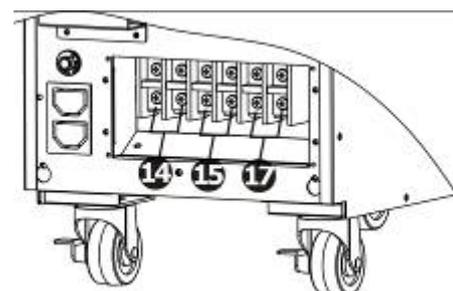
Diagram 2: 6K(L)/10K(L) Input/Output Terminal
