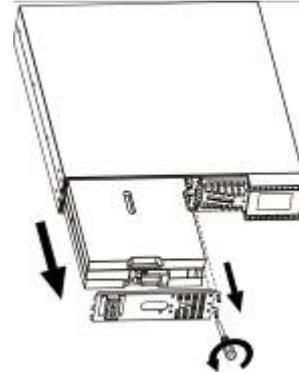
Pull out the battery box by removing two screws on the front panel.
