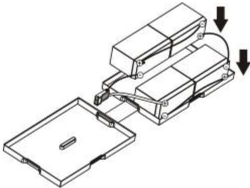
Step 4: Cover the other side of plastic shell as below chart. Then, battery kit is assembly well.
