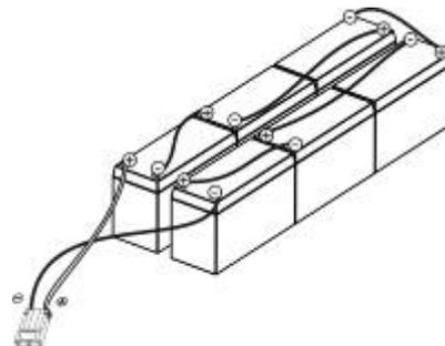
Step 3: Put assembled battery packs on one side of plastic shells.
